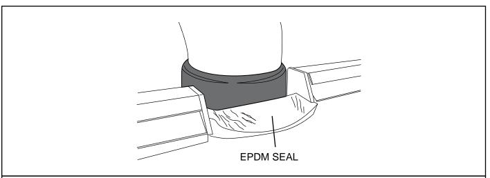
**14.** Cut the EPDM seal to required length and seal the gaps near the sports bar foot.
