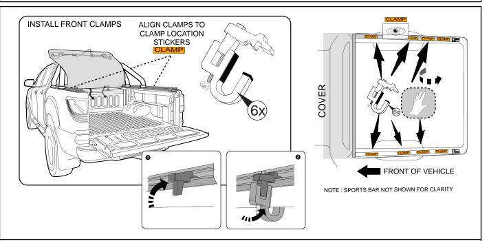
**10.** Using the clamp location stickers on the side rails, mount front clamps to the tub body ensuring that the side rails are flush with the outside of the tub body.
