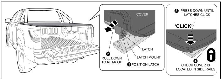
**16.** Position latches into stretch mounts. Holding the cover rail at the rear, roll towards the rear of the vehicle and down until latches click and are both locked into position. Ensure the flexible side flanges are fully seated into the side rails.
