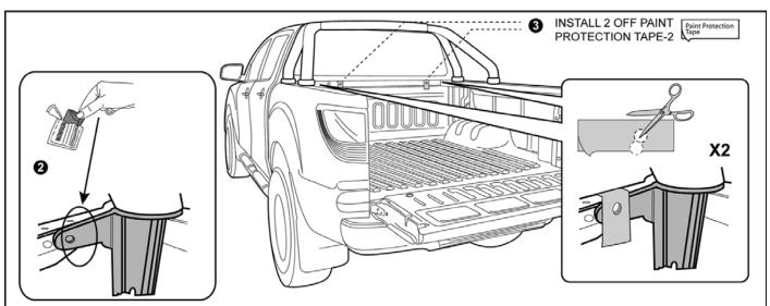
3. Make a clearance hole in the paint protection tape-2 (2 off). Clean the tub/sportsbar bracket area with alcohol wipes, align the holes in the paint protection tape with holes in the sportsbar bracket as shown in diagram above and apply tape.
