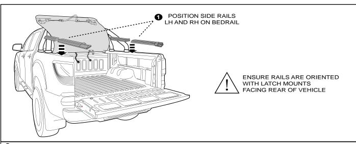
**8.** Position Side Rails on the tub sides ensuring latch mounts are orientated to the rear of the vehicle.
