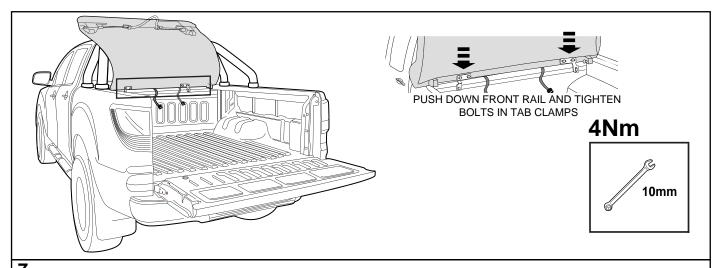
7. Align the Tonneau with the sports bar front legs, push down the front rail and tighten bolts in tab clamps.
