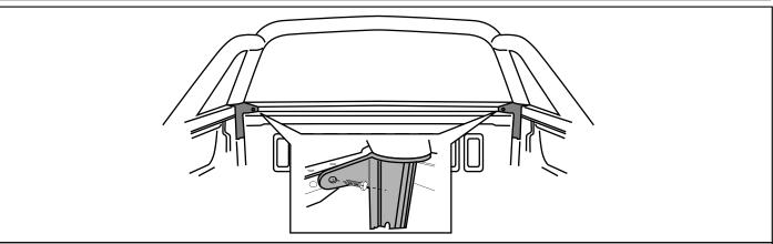
1. Remove the existing sportsbar bracket front screw (2 off). Note:Do not remove the sportsbar bracket screws on the sides.
