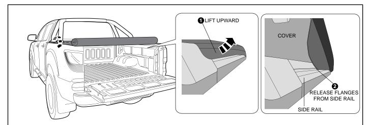
**2.** Working from the rear of the cover, grip and lift in an upward direction to release the flexible flanges from the side rails
