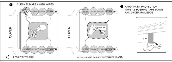
**9.** Clean the tub areas with alcohol wipes in the location marked 'CLAMP' on the side rail and apply the paint protection tape -2 (16 off).
